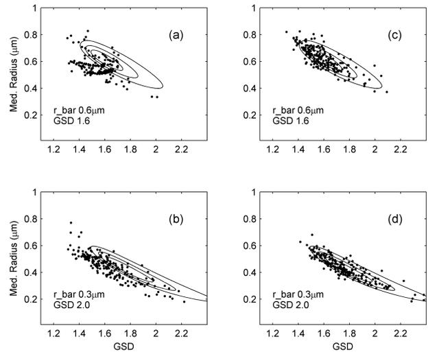
Fig. 2. Scatterplots of forward Monte Carlo outcomes with contours of Bayesian PDFs. Outcomes using MMD retrievals are shown in (a) and (b). MPPDF retrievals are shown in (c) and (d). The modeled true distribution parameters,  $(\bar{r}, \sigma)$ , are (a), (c)  $(0.6 \mu\text{m}, 1.6)$ , [corresponding to Figs. 1(a) and 1(e)], and (b), (d)  $(0.3 \mu\text{m}, 2)$ , [corresponding to Figs. 1(d) and 1(h)].
