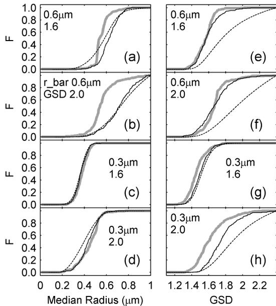
Fig. 1. (a)–(d) CDFs of retrieved median radius and (e)–(h) GSD with modeled true distribution parameters  $(\bar{r}, \sigma)$  of: (a), (e)  $(0.6 \mu\text{m}, 1.6)$ ; (b), (f)  $(0.6 \mu\text{m}, 2)$ ; (c), (g)  $(0.3 \mu\text{m}, 1.6)$ ; (d), (h)  $(0.3 \mu\text{m}, 2)$ . The dotted curves represents the Bayesian posterior CDF. The thin black curves represent the estimated CDF using MPPDF retrievals. The thick gray curves represent the estimated CDF using MMD retrievals.
