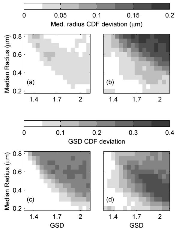
Fig. 3. (a), (b) Median radius and (c), (d) GSD CDF deviation from the Bayesian CDF as formulated in (29) using the (a), (c) MPPDF and (b) (d) MMD retrieval methods.
