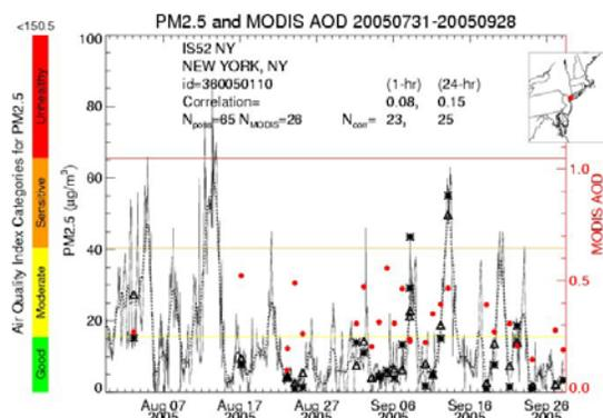
Fig. 1 IDEA matchup between measured PM2.5 and the MODIS estimator based on a static aerosol PBL model.
