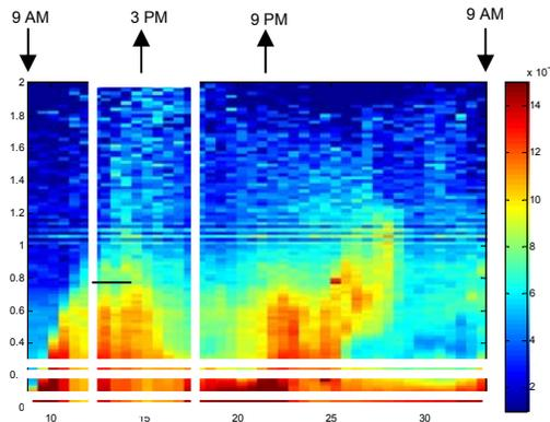
Fig 2 36 Hour Ceilometer measurements of near surface backscatter
