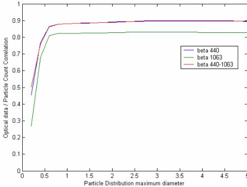
Fig 1 Correlation between partial volume and optical backscatter as function of upper diameter limit.
